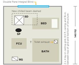
**Corridor side:** Lay-in ceiling with primary air, CHWS/R and HHWS/R mains with branch piping to FCU, 2-way control valve
